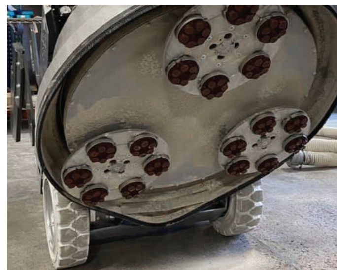
Left to Right: L20GEB with Quick Change SA Metals; L38GREB with Calibra pucks on Lippage Holders
